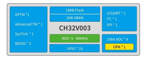
The muNico board provided by AtrivaTech utilizes the F4 P6 version of the CH32V003 which is fully compatible with existing opensource software development kits and specialized software CH32V003FUN by Charles Lohr and Arduino IDE plugin provided by WCH themselves.
